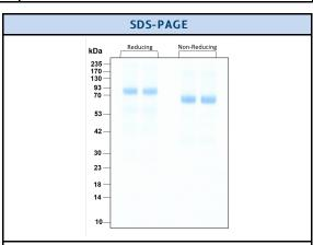
Purity of GMP-grade recombinant human HGF was determined by SDS- polyacrylamide gel electrophoresis. The protein was resolved in an SDS- polyacrylamide gel in reducing and non-reducing conditions and stained using Coomassie blue.
